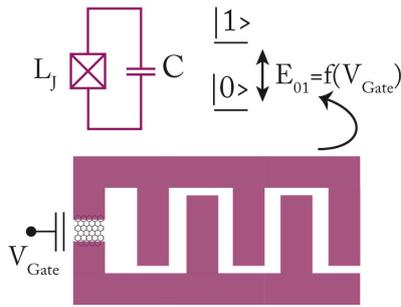
**Figure 1: the equivalent electrical circuit shows that this device will behave as an electrically tunable quantum two-level system.**
