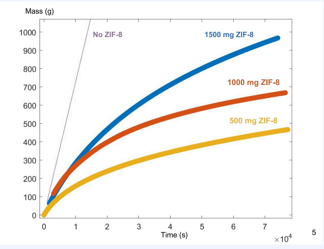
Non linear evolution of the flowrate demontrates the formation of a compact deposit that does not tend to stabilisation.
