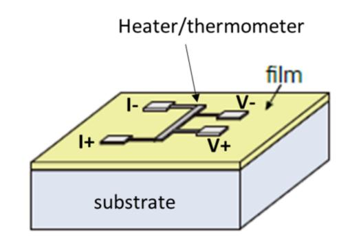
$$\Delta T = \frac{2V_{3\omega, \text{rms}}}{R_{e,0}I_{1\omega, \text{rms}}\beta}$$
