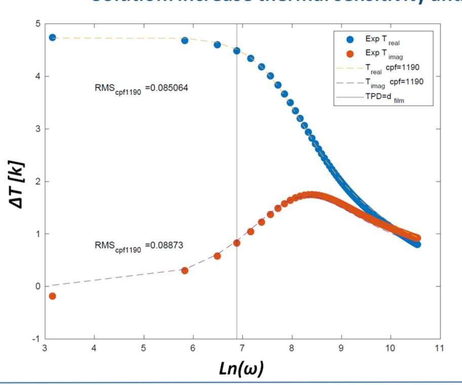
Model fitting is good both for real part and imaginary part of temperature oscillation. But...
