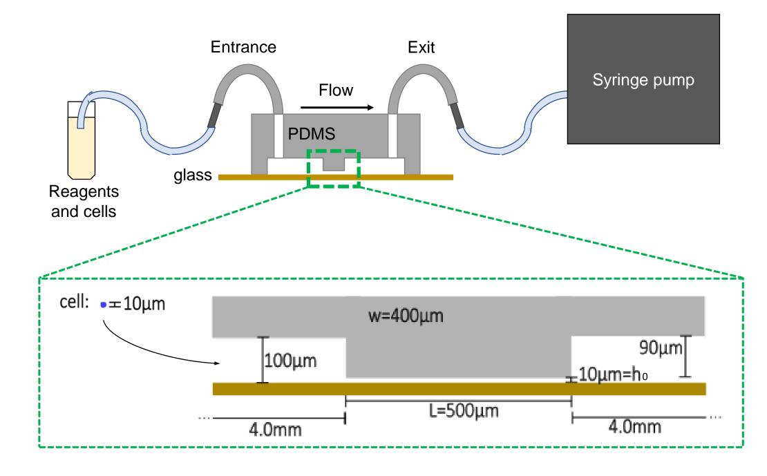
To impose the physiological conditions of the microcapillaries, the microfluidic channel has a thin region  $(h_0, L, w)$  with a similar size than cells (~10µm)
