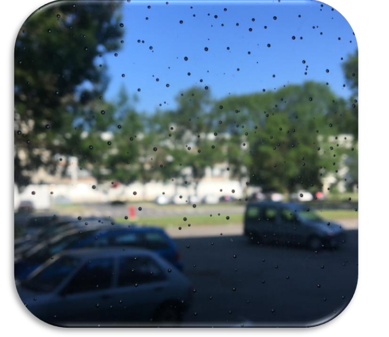
1. Bubble in laminated glass. Taken by Claire Schune.
